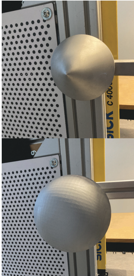
Figure 43: Alignment target fixed for robot mounted camera, top: alignment cone, bottom: alignment sphere
